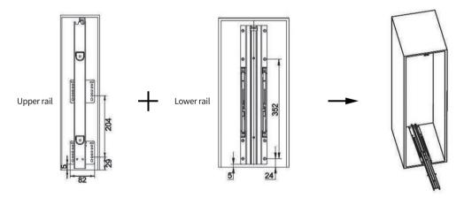
2. As shown in the figure, put the plug into the main frame, and then fix the main frame with holes into the cabinet, and connect it to the upper and lower rails. Lock the screws through the corresponding screw holes.
