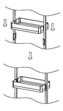
6.Complete the installation, pull back and front to test whether the guide rail is smooth.
