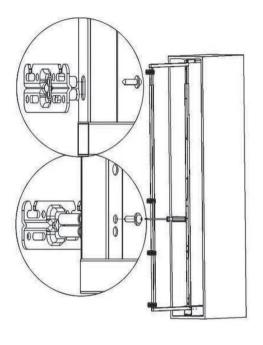
4. According to the figure below, lay the door panel flat, fix the door panel with the door panel connect1on, adjust the positioning hole, and lock the screw.
