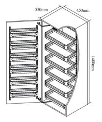
5) Hanging small and large basket on the frame, finished install, the reveal can open and close freely.
