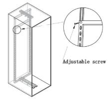
3) Adjusting the height of mainframe with adjustable screw, and installing it on the inside cabinet.
