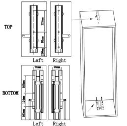
1) Installing up and down slide as picture show.
