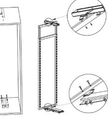
2) Look frame on the connector of the up and down slide with screw as the picture show.
